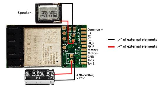
Connection of additional external elements (servos, digital couplings)
