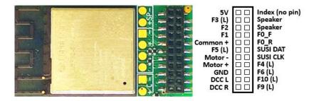
Connection of basic external elements (speaker and capacitor)
