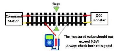
**Important**: The transition voltage between the Booster ranges should be less than 0.8 V. This can easily be checked with a multimeter (setting the measuring range to AC alternating voltage). Both rails gaps should always be checked. If the value of 0.8 Volt exceeded, then input voltage of the booster or the voltage setting of the Command Station must be adjusted.
