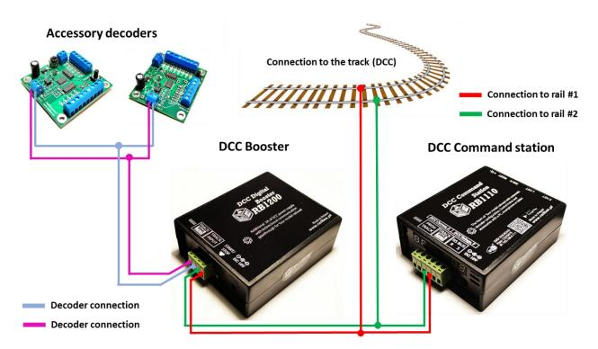
**Note:** DCC Booster RB 1200 can also be used as supplying source for any of your accessory decoders.
